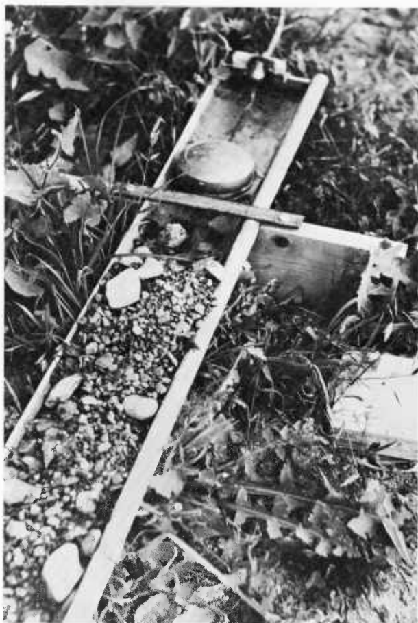
FIGURE 2.—Four-inch eaves trough filled with coarse gravel and equipped with float water-level control.
